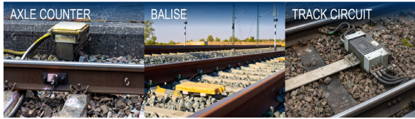
Figure 1: Cost-intensive trackside detection equipment
